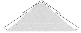
Field-Form a Two-Piece Flashing (Can Be One-Piece with Precise Measuring)
