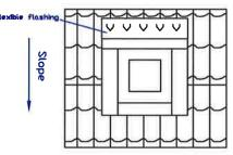
Install flexible flashing over the back flashing and over the ribs on the panel.
