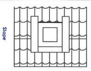
The side flashings should extend over the front flashing and up the sides of the chimney.
