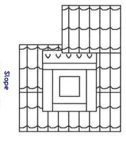
Install the next course of panels over the flexible flashing.
