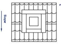
The back flashing should extend up the chimney, over the side flashings, and over the panels. Some of the high spots in the panel may need to be removed to allow the flashing to rest as flat as possible.
