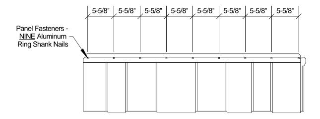
Section Plan View Nail Pattern Assembly
