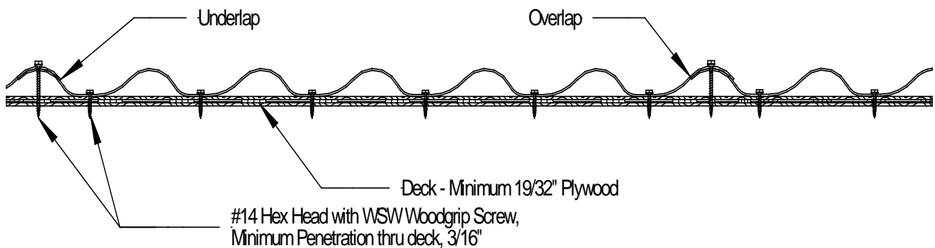
Detail "2A" - Assembly Profile View (Typical Fastener Pattern Across Alternate ODD Rows)
